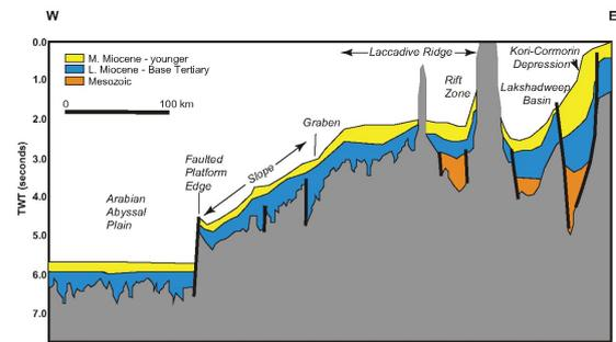
Figure 6. Tracing of multi-channel seismic line from the Kerala-Konkan-Lakshadweep (KKL) basin extending southwest into the Arabian Abyssal Plain (Location on Figure 4, modified from Scaife, 2012). The inferred age interpretation of the sedimentary section is shown in Orange (Mesozoic), Blue (L. Miocene - Base Tertiary), and Yellow (M. Miocene- younger). The total sedimentary thickness shown is 3 seconds of Two-way Time (approximately 3 km or more). Further details in text.
