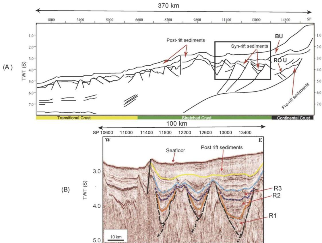
Figure 5. Multi-channel seismic line from the Mumbai offshore basin extending southwest into the southern edge of Laxmi Basin. Location shown in Figure 4. ROU is Rift-onset unconformity. BU is Break-up unconformity. See descriptions of R1, R2, and R3 sequences in text. Blue line in 5B marks the boundary between syn-rift and post-rift sediments. Yellow horizon is interpreted as middle-Miocene in age (modified from Pandey and Pandey, 2015).
