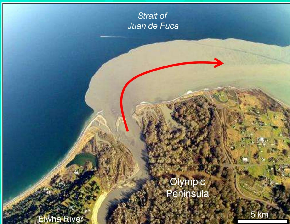
Sediment plume triggered by Elwha Dam demolition in the State of Washington
